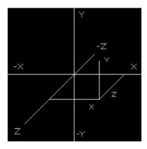
The viewing volume is the volume or area that a 3D object can be rendered in and be seen by the viewer. Think of the viewing volume as a 4 sided pyramid with the top tip at 0, 0, 0 and the body of the pyramid extending in the negative Z direction. The viewer's eye is located at the top tip of the pyramid and is looking into the body of the pyramid.
